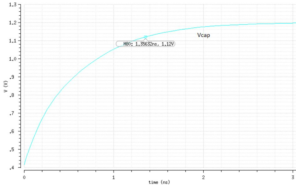
Figure A.2: Capacitor's charging from the value 1 to 3
