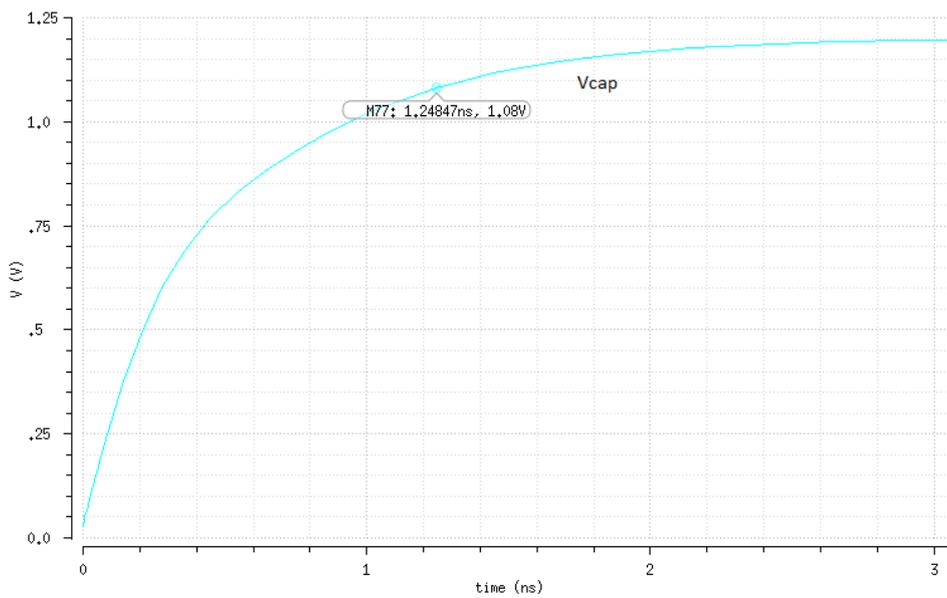
Figure 4.3: Capacitor's charging from the value 0 to 3
