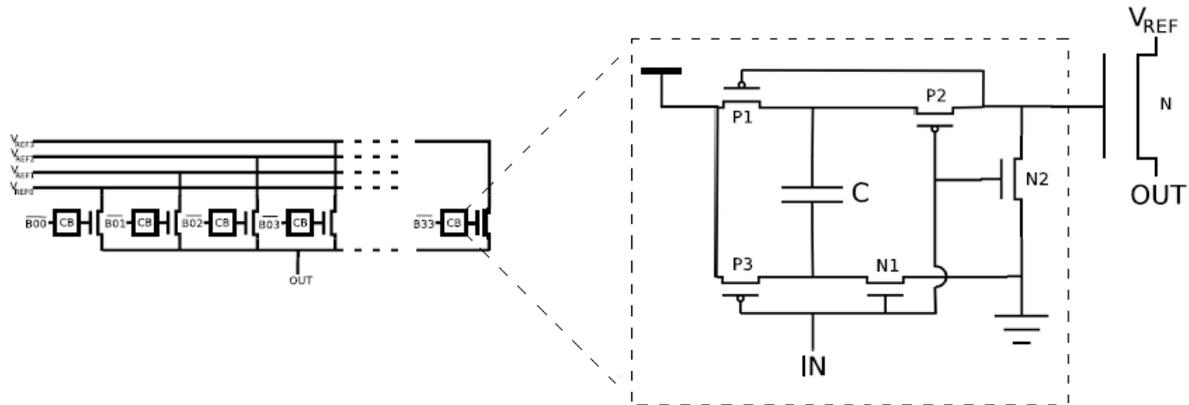
Figure 2.4: Multiplexer block diagram and clock boosting circuit schematic
