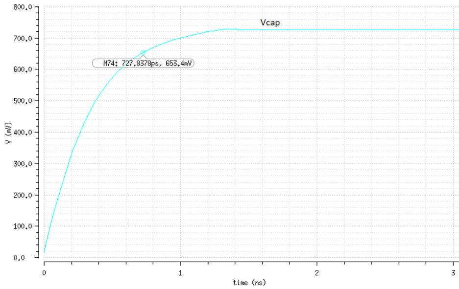
Figure 4.2: Capacitor's charging from the value 0 to 2
