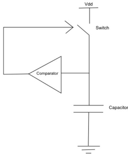
Figure 3.2: Simplified voltage generator block diagram
