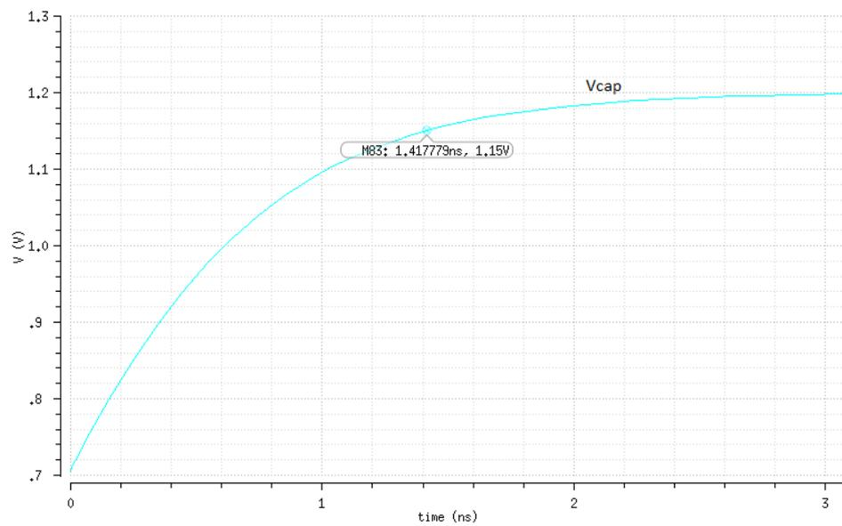
Figure A.3: Capacitor's charging from the value 2 to 3
