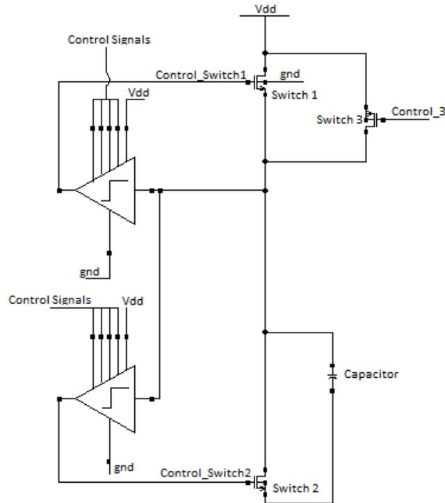
Figure 3.4: Qlut with voltage generator block diagram
