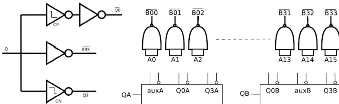
Figure 2.2: Q-decoder logic block diagram
