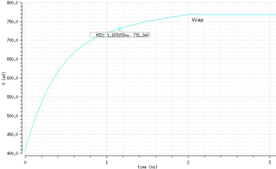
Figure A.1: Capacitor's charging from the value 1 to 2
