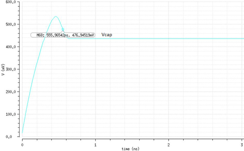
Figure 4.1: Capacitor's charging from the value 0 to 1
