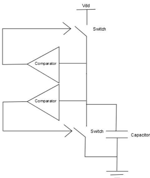
Figure 3.3: Simplified voltage generator block diagram with discharge circuit
