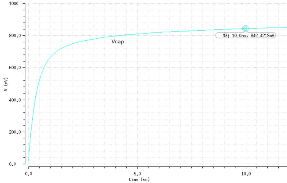
Figure 3.7: Charging of a comparator using a voltage follower NMOS switch
