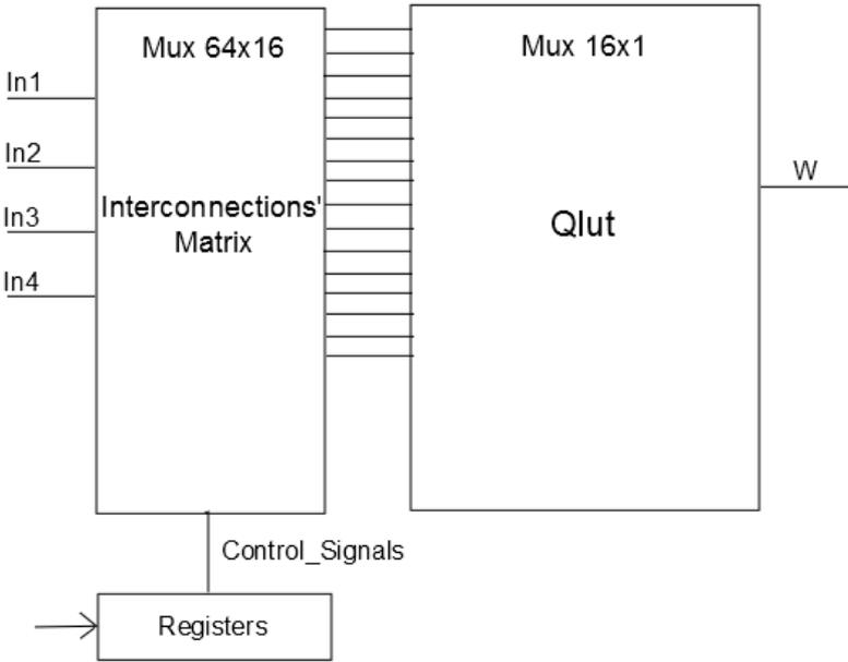
Figure 3.1: Simplified interconnection's matrix block diagram
