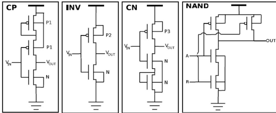
Figure 2.3: CP, INV, CN and NAND logic gates schematics
