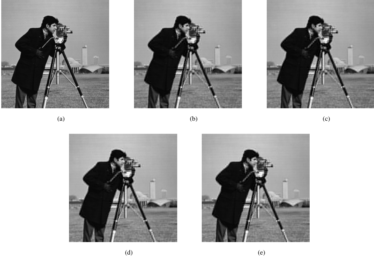
Fig. 4. (a) Original cameraman image; Its compressed versions using: (b) original DCT matrix; (c) optimized DCT matrix when \epsilon_1 = \epsilon_\infty = 4 ; (d) optimized DCT matrix when \epsilon_1 = \epsilon_\infty = 8 ; (e) optimized DCT matrix when \epsilon_1 = \epsilon_\infty = 16 .
