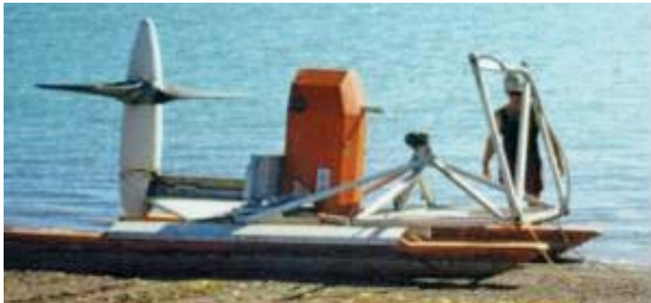
Figure 5 The NTU – NT PAWA Kinetic tidal energy converter, on shore for maintenance
